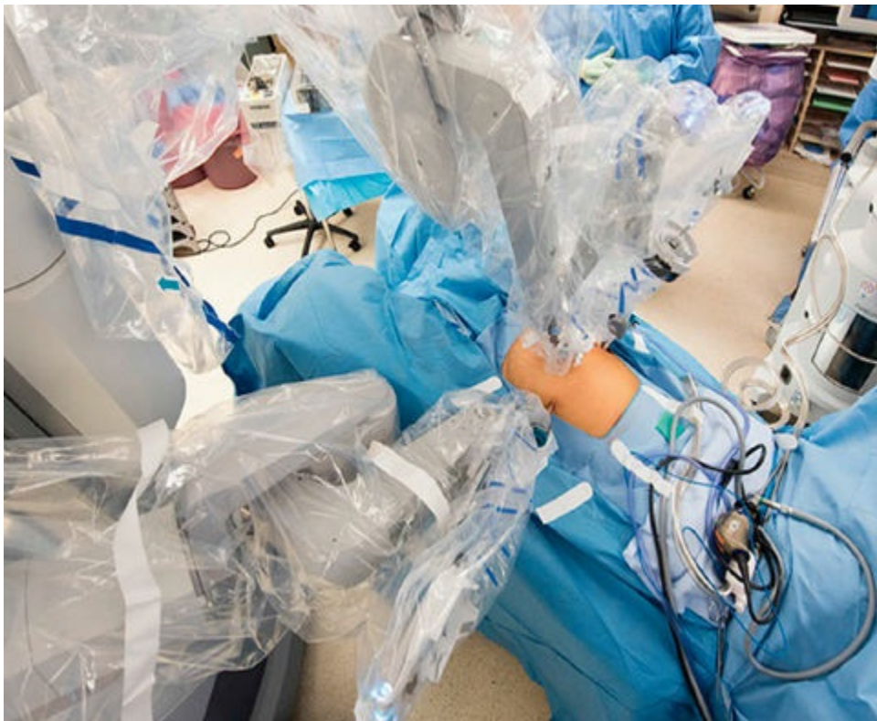
Tech Figure 7.3.4. Picture of robotic ports and placement of robotic arm over trocar.
