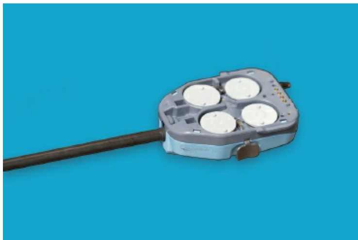
Figure 2.10. Flat side of the instrument housing unit—which interfaces with the robotic arm sterile adapter. Robotic instrument release lever (one of two) on the side of the
