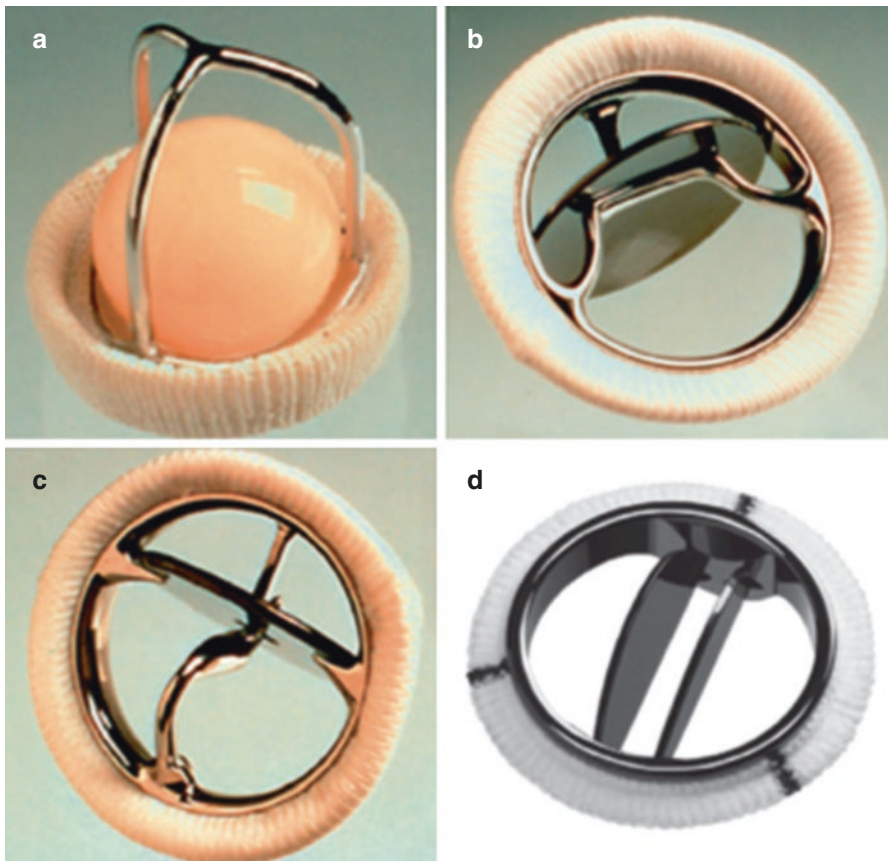
Fig. 35.1 Examples of mechanical heart valves. (a) Starr-Edwards caged-ball valve which is associated with the highest thrombogenicity. (b) Bjork-Shiley tilting-disk valve is an example of a tilting-disk valve which has intermediate risk of thrombogenicity. (c) Medtronic Hall tilting-disk valve. (d) St. Jude Medical Regent is an example of a bileaflet valve which has the lowest risk of thrombogenicity. Reprinted with permission from Lancet. 2009;374:565–76
