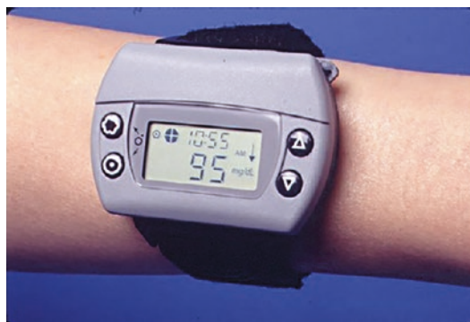
Fig. 6.7 The GlucoWatch G2 Biographer developed by Cygnus, Inc. (USA), and approved by the FDA in 2001 was a glucose monitoring device which allowed non-invasive glucose monitoring through the skin (Image kindly provided by and with permission from Dr. R. Potts)
