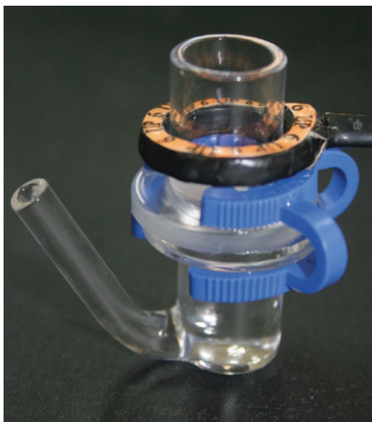
Fig. 12.3 Dermaportation coil mounted on a Franz diffusion cell
