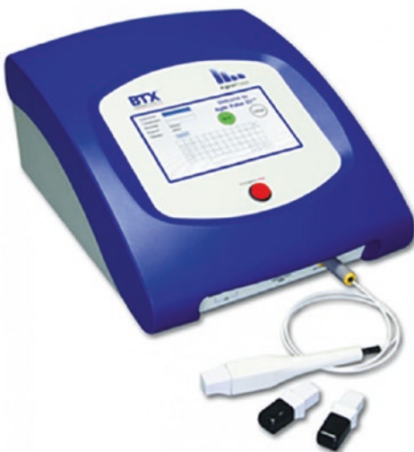
Fig. 8.3 Agile pulse in vivo system from BTX® Instrument Division, Harvard Apparatus Inc., USA, for intradermal vaccine and gene therapy (Reproduced with kind permission from Harvard Apparatus Inc., USA)
