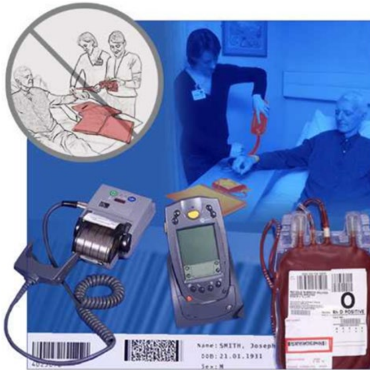
Figure 23.3 Bedside checking using an electronic system. The traditional method of pretransfusion bedside checking requires two nurses and checks of multiple items of written documentation. With barcode technology, a handheld computer reads a barcode on the patient wristband containing full patient details. The handheld computer checks that the patient details on the wristband barcode match those on the barcode (in the red box) on the compatibility label attached to the unit after pretransfusion testing. This barcode also contains the unique number of the unit, and is matched with the barcode number of the unit (top left of the bag) to ensure that the blood transfusion laboratory has attached the right compatibility label. Source: Reproduced with permission from Wiley–Blackwell. (See insert for colour representation of the figure.)
