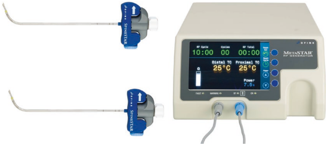
Fig. 2.5 The STAR Tumor Ablation System consists of the MetaSTAR generator and the SpineSTAR ablation instrument (Courtesy of DFINE, Inc.)
