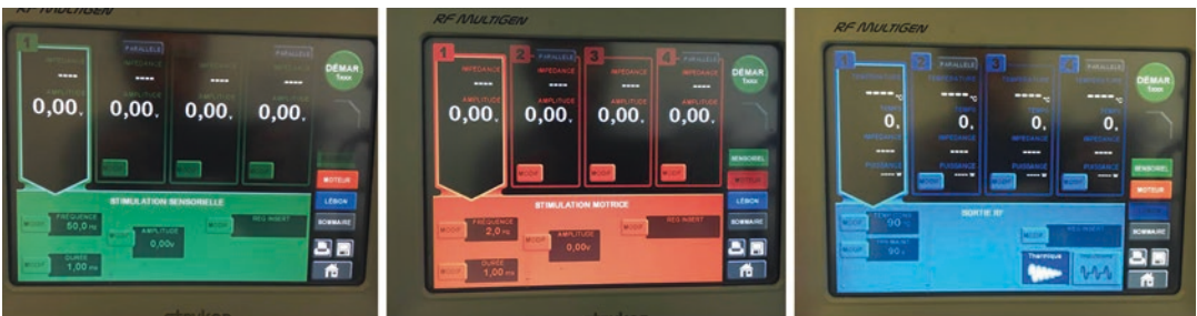
Fig. 6.7 The generator's screen as it appears during motor and sensory stimulation tests as well as during continuous thermal ablation mode
