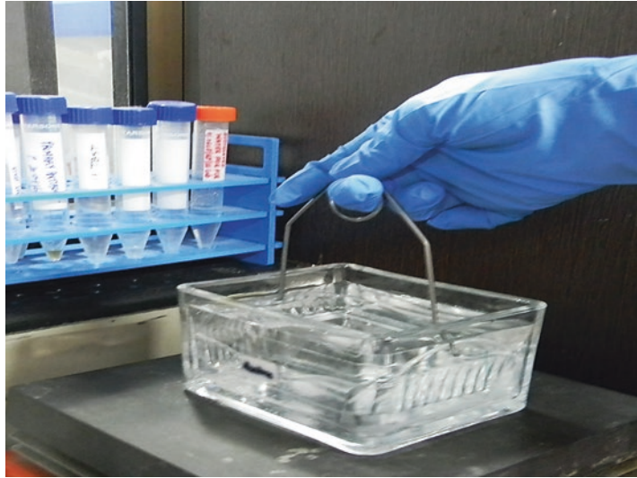
Fig. 5 The slide is placed in the Wheaton glass chamber and rinsed with 1× TBST using a magnetic stirrer
