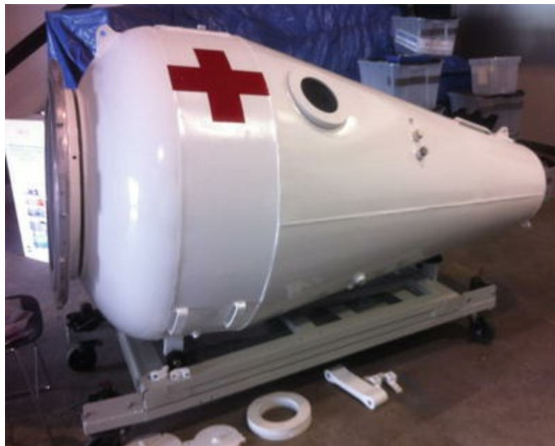
Fig. 42.21 An example of an EMS transport chamber which would admit the patient and paramedic in transport to a hospital-based unit from an event on the street; the ambulance would need no
