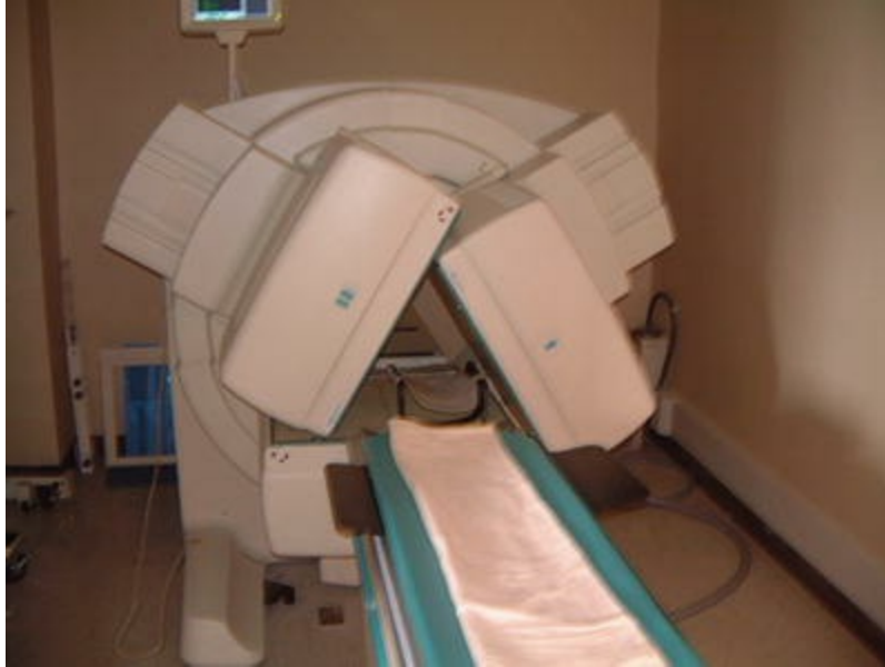
Fig. 10.2 Example of SPECT brain imaging device with three imaging “heads” that slowly revolve around the patient’s head during the 20-min scan
