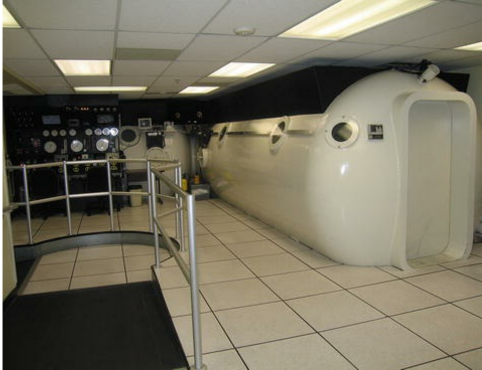
Fig. 7.5 OxyHeal 4000 Class A Multiplace hyperbaric chamber. A 3-lock, 6 ATA, 18-patient horizontal cylinder hyperbaric chamber system at Presbyterian/St. Luke's Hospital in Denver, Colorado, USA. This chamber performs a significant number of critical care treatments annually. Photo courtesy of OxyHeal Health Group, La Jolla, CA 92038, USA
