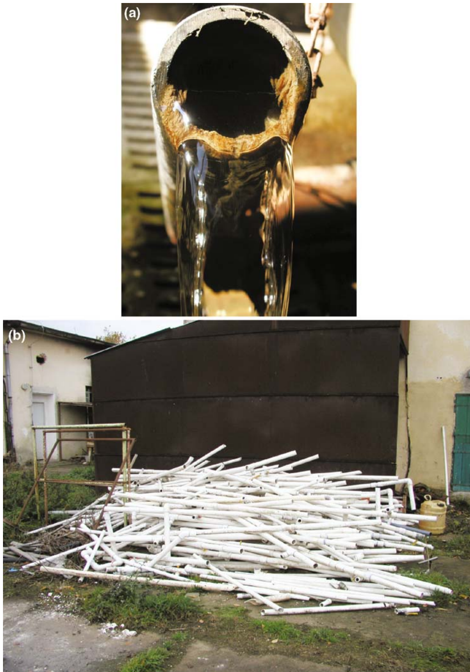
Photo 3.3 Biofilms can increase rapidly in number in pipelines through which highly organically polluted water flows (tanks for fresh water fish aquaculture are supplied with surface water) (a). In biofilms, both M. kansasii and other mycobacterial species with consequences for health have been detected; these can multiply in this environment if the temperature is convenient (Chapter 4). Water contaminated with released biofilms or freely floating mycobacteria can pose a risk to host organisms and feeds, foods, the aquarium environment, fish present in the aquarium and other animals, etc. It was discovered on a pig farm that plastic water piping was a source of ESM and PPM (b). In the summer months, water became warm there relatively quickly due to its better heat conductivity in comparison with metal piping. The surface of the plastic material evidently facilitated the production and subsequent persistence of biofilms on the piping walls. After the occurrence of tuberculous lesions caused by various species, especially PPM including M. kansasii , in the head and mesenteric lymph nodes of pigs, the breeder was forced to exchange the plastic for metal piping (Photo I. Pavlik)
