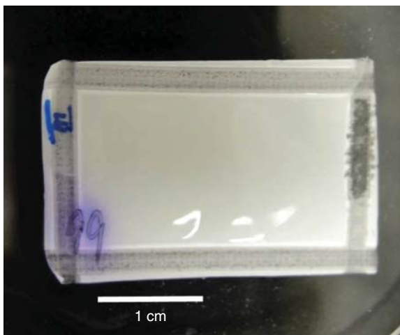
Figure 17.3 Macrocapsule device constructed using a semipermeable biocompatible polymeric membrane. Scale bar: 1 cm.
