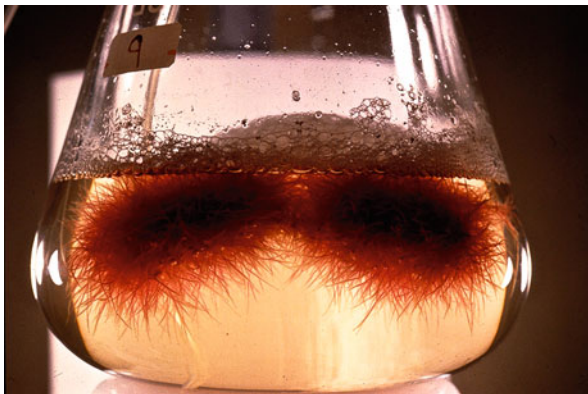
Fig. 12 Red beet roots transformed by wild type A. rhizogenes in an early stage of culture with aeration by sterile air pumped through an aquarium stone. Bioreactors are not needed to grow transformed roots. Cultures can be aerated with simple aquarium equipment plus a filter to sterilize incoming air, and the pressure produced is sufficient to remove medium for extraction and renewal. In one such culture, morning glory root density was so high that they had to be sawed to remove them from the culture vessel and the aquarium stone was never found, apparently digested by the roots (Photo D. Tepfer)
