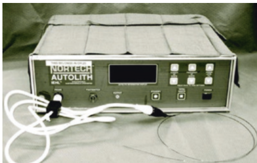
FIGURE 11.12 Electrohydraulic lithotrite (note the miniaturized flexible probe). Reproduced from Miller J and Stoller ML [89] with permission from Springer
