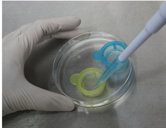
Fig. 3 Collecting the organoids for CTOS isolation. The 100 µm cell strainer ( yellow ) and 40 µm cell strainer ( blue ) are dipped in 30 mL HBSS in a 10 cm tissue culture dish. The fragments that remain in the cell strainer are collected with a 1 mL micropipette
