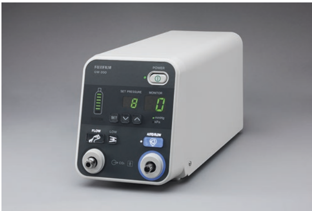
Fig. 23.1 Computer-mediated automatic insufflation unit for flexible GI endoscopy (GW-200, Fujifilm Corporation, Tokyo, Japan)
