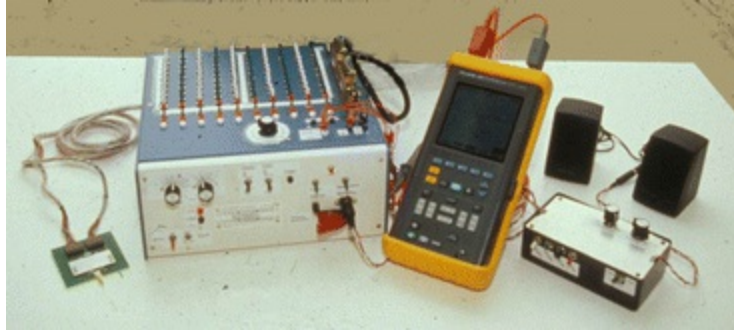
Fig. 7.3 The portable, battery powered stimulation system used in our acute human trials. The blue and white box is the 100-channel stimulator, connected via a 7-ft cable to a green circuit board containing the electrode array (at left). A portable battery-powered oscilloscope monitors the voltages, and a set of speakers creates a tone to alert the subjects to the timing of the stimulus
