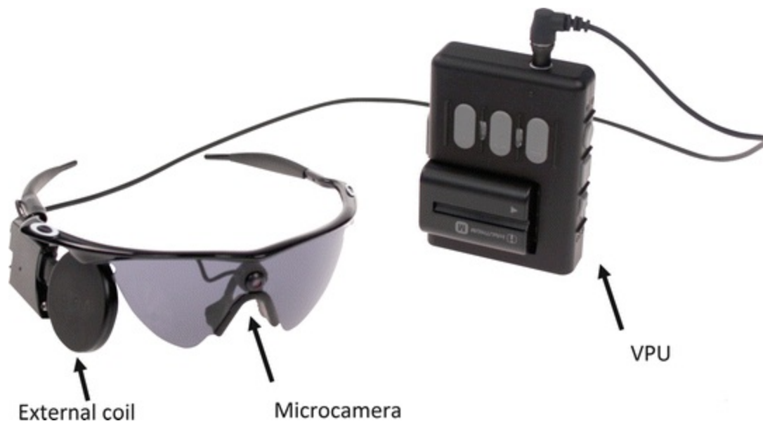
Fig. 5.2 Photograph of the Argus® II retinal prosthesis system showing the glasses-mounted microcamera, the external (inductive) coil and the video processing unit (VPU) (Reprinted with permission from Second Sight Medical Products, Inc.)
