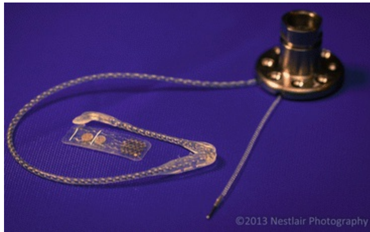
Fig. 10.2 The clinical suprachoroidal electrode array ( left ) and percutaneous lead system ( right ) used for research purposes in the initial BVA pilot study (2012–2014) (Courtesy of Dr. David Nayagam, Bionics Institute Australia)
