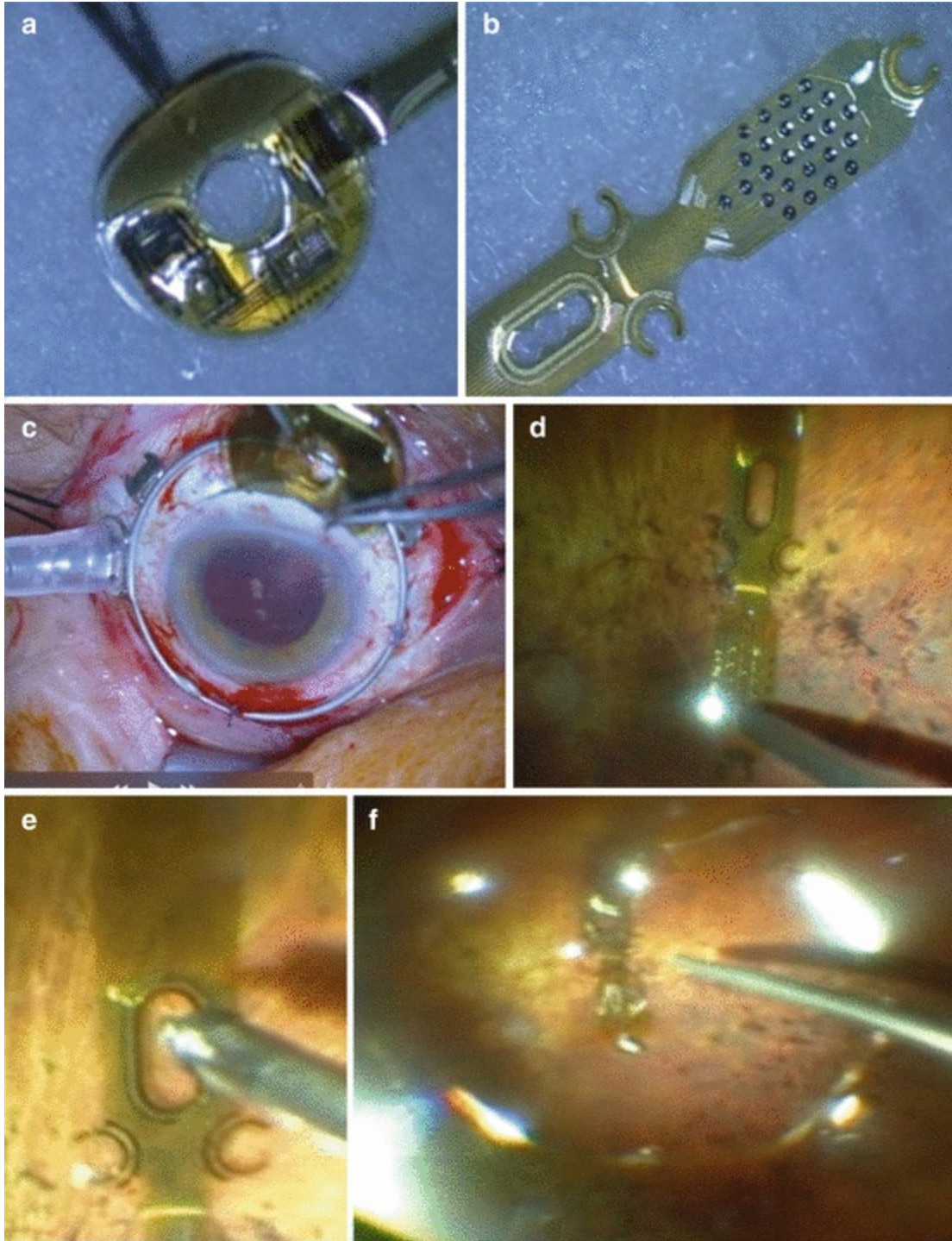
Fig. 12.3 Major steps of the EPIRET implantation. (a) Semiflexible receiver system with microfabricated coil and two microASICS for signal extraction and pulse generation. (b) Stimulator head with 25 IrOx electrodes on a polyimide base. (c) Insertion of the receiver lens through a 11 mm corneoscleral incision in the posterior chamber. The eye is stabilized with the pp infusion and an additional Fliringa ring. (d) The stimulator head is positioned onto the central retina using a soft tip fluid needle. (e) Fixation is done with a standard retinal tack. (f) The eye is closed after fluid air exchange
