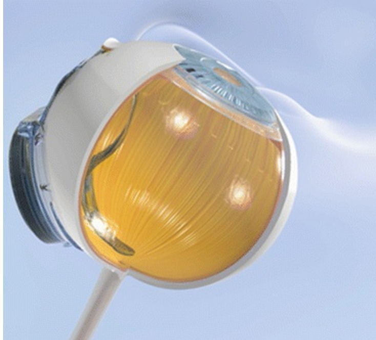
Fig. 8.5 Extra- and intraocular part of the IRIS implant
