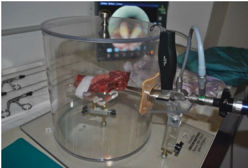
Fig. 8.14 The polycarbonate allows constant verification of the accurate placement of the specimen, the laryngoscope, and instruments during training
