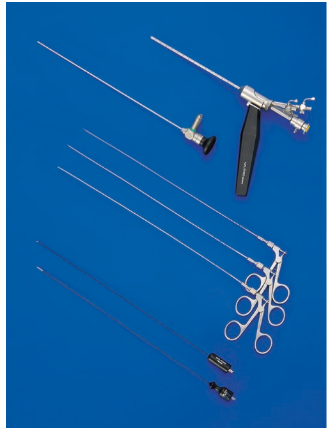
Fig. 2.28 Oi HandyPro system, with removable handle, including operating sheath handle (three work channels), mandrel, and wide-angle straightforward telescope 0° (enlarged view, diameter 2 mm, length 26 cm). Instruments (diameter 1.3 mm, working length 30 cm), including scissors (single-action jaws), biopsy forceps (double-action jaws), grasping forceps (double-action jaws), unipolar coagulation electrode, and bipolar coagulation electrode (Images courtesy of Karl Storz, Tuttlingen, Germany)
