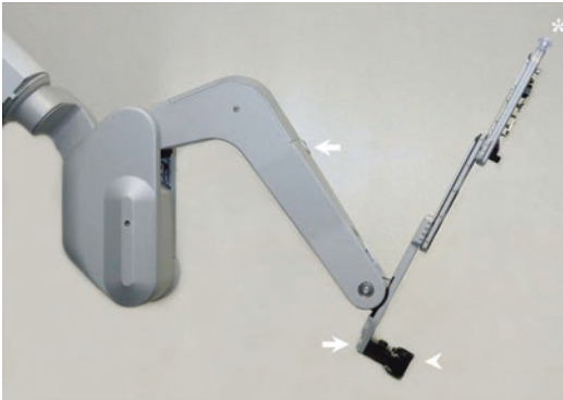
Fig. 3.14 Photograph of the da Vinci® S and HD instrument arm showing the port clutch buttons ( arrows ) and
