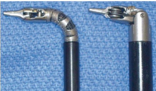
Fig. 3.20 Photograph of EndoWrist ® needle drivers. On the left is a 5 mm needle driver with the “snake joint” compared to the 8 mm needle driver with an “angled joint”
