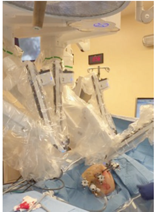
Fig. 11.20 The Da Vinci Xi system has an overhead arm base that allows for improved trocar positioning and multi-quadrant operation
