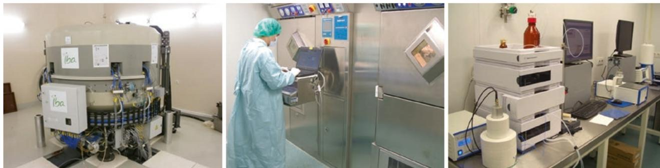
**Fig. 10.1** From left to right: an open horizontal cyclotron, radiopharmaceutical synthesis laboratory, and RP quality control laboratory
