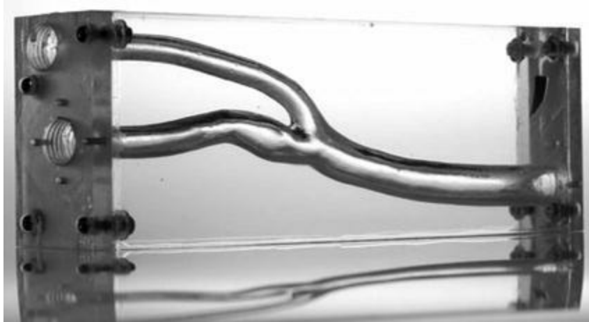
Fig. 12.7 Carotid artery bifurcation rigid flow phantom. The phantom is for use in optical studies manufactured using the ‘lost core’ approach. From; Experiments in Fluids; Fabrication of rigid and flexible refractive-index-matched flow phantoms for flow visualisation and optical flow measurements ; Vol. 52, 2012, pp. 1331–1347, Geoghegan P, Buchmann N, Spence C, Moore S, Jermy M; © Springer-Verlag 2012, with permission of Springer
