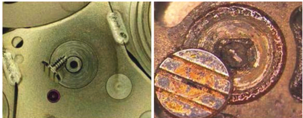
Example of component damage of motor assembly screws due to corrosion.
