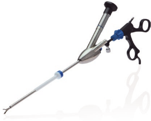
Fig. 29.2 Operating scope Set “Leipzig Egg” (Richard Wolf GmbH, Knittlingen, Germany) possess a 5.5 mm Operating scope with a 3.5 mm working channel and a 0^\circ direction of view 0^\circ , and working length of 215 mm (Image: Courtesy of Richard Wolf GmbH, Knittlingen, Germany)
