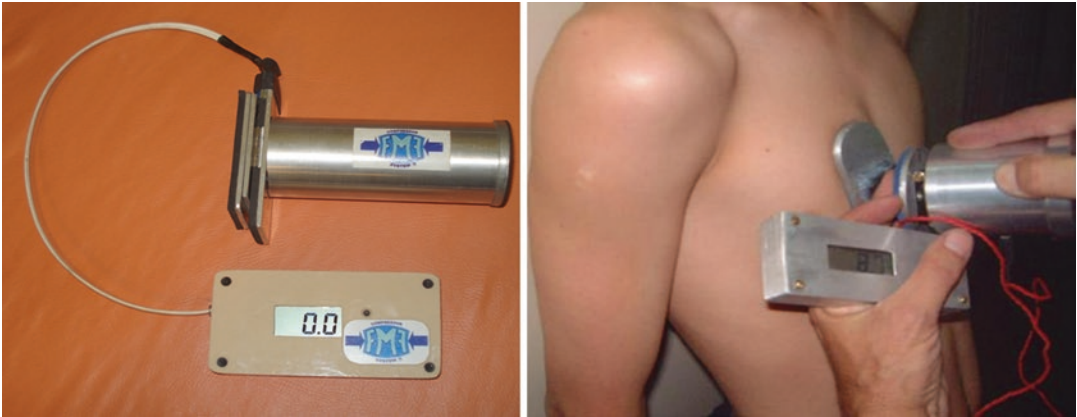
Fig. 46.6 Left: Early version of the electronic PMD used to measure the PIC in PSI units. Right: The same device compressing the defect of a patient with PC during inspiration
