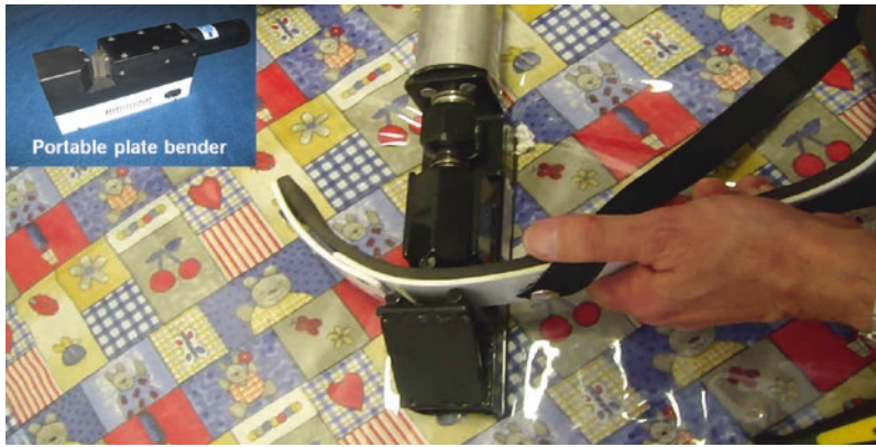
Fig. 46.12 Portable plate bender to model lightweight aluminum curved segments during consultation
