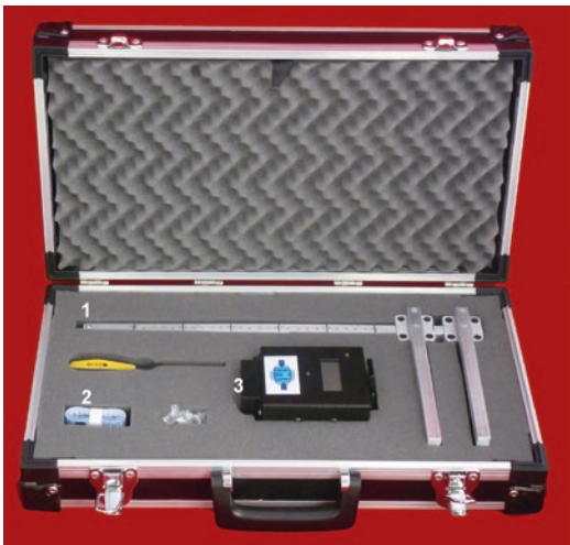
Fig. 46.15 Briefcase with the instruments and materials required to obtain the standardized measurements to order the brace. Ref: (1) chest measuring ruler, (2) metric tape, (3) PMD. It includes a screwdriver and screws, too
