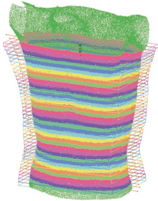
Fig. 17.12 Transverse slices among which the most deformed slice is searched (open slices have been neglected). Different colors apply to different slices
