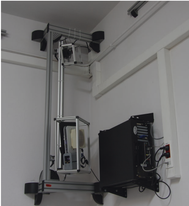
Fig. 17.3 The components of the measurement system as installed in a laboratory at Medical University of Warsaw: a modified DLP projector at the bottom, a CCD camera at the top and a PC at the side
