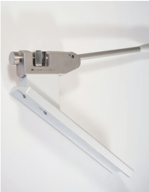
Fig. 26.4 Orthopedic plate bender press to bend the pectus bar (Courtesy: Hofer GmbH, Fürstenfeld, Austria)
