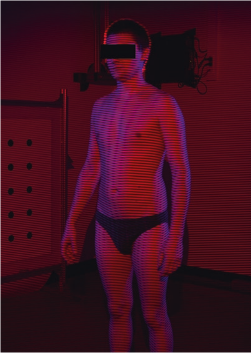
Fig. 17.5 Healthy subject's body covered with red and blue sinusoidal fringes projected during the measurement
