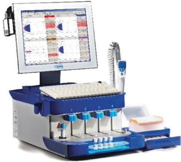
Fig. 11.5 Photograph of the ROTEM® delta hemostasis analyzer (Used by permission of Tem international GmbH)
