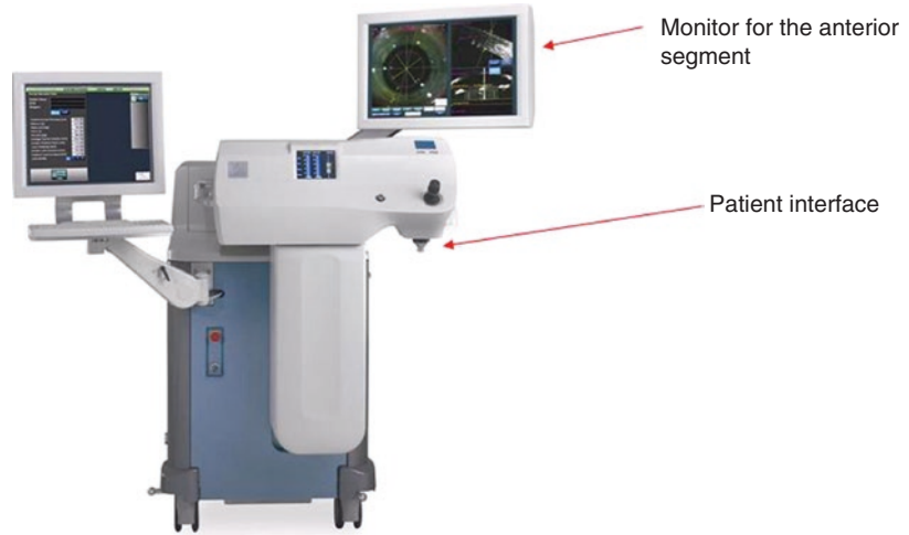
Fig. 7.1 The Alcon-LenSx femtolaser. The left monitor is for to set the treatment parameters, the right LCD monitor helps the surgeon throughout the femtolaser treatment, underneath the patient interface (PI) which comes into contact with the treated eye
