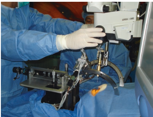
Fig. 14.4 Intraocular Robotic Interventional Surgical System (IRISS) working prototype (Image courtesy of JP Hubschman)
