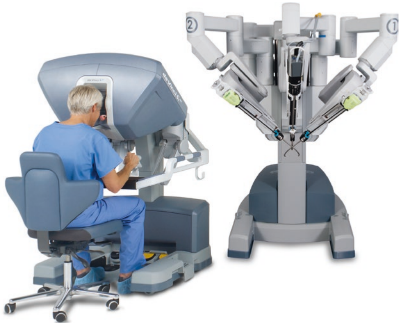
Fig. 14.1 Da Vinci Surgical System showing surgeon looking into console viewer, robot with arms separated physically from surgeon's console (Image courtesy of Intuitive Surgical)
