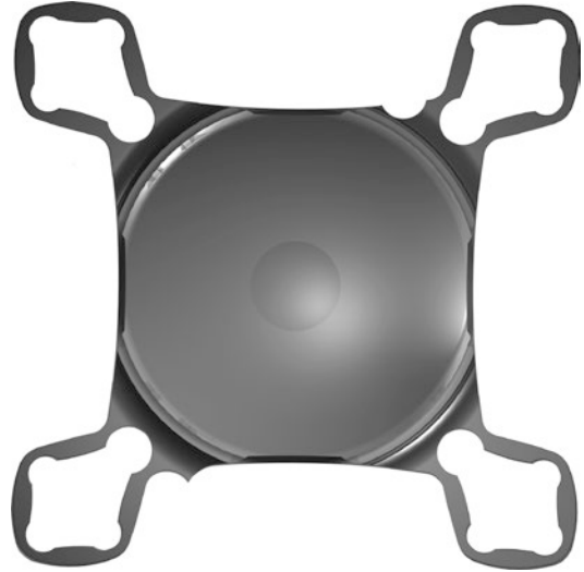
Fig. 10.1 Image of Scharioth Macula Lens (Medicontur Hungary Ltd. Hungary), lens design is based on A4 W add-on IOL (1stQ, Germany), note central optical portion of 1.5 mm diameter with +10.0 diopters, residual optic is optically neutral and has a diameter of 6.0 mm, overall diameter is 13 mm, lens is made from hydrophilic acrylic material and requires a minimum incision size of 2.2 mm if implanted with injector
