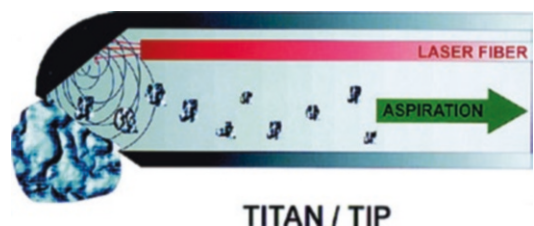
Fig. 8.1 The titan tip of a nano laser (ARC, Germany). The laser induces a plasma and shock wave and disrupts the nucleus. The nuclear material is aspirated through the same needle
