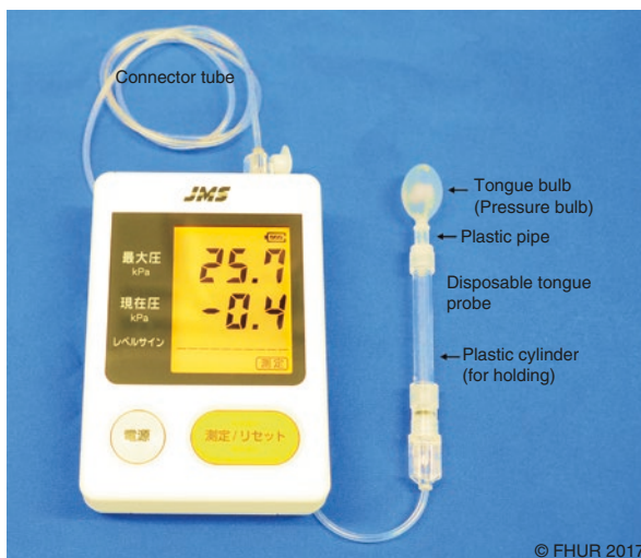
Fig. 5.56 Balloon-type tongue pressure measurement device (JMS Co. Ltd., Hiroshima, Japan)
