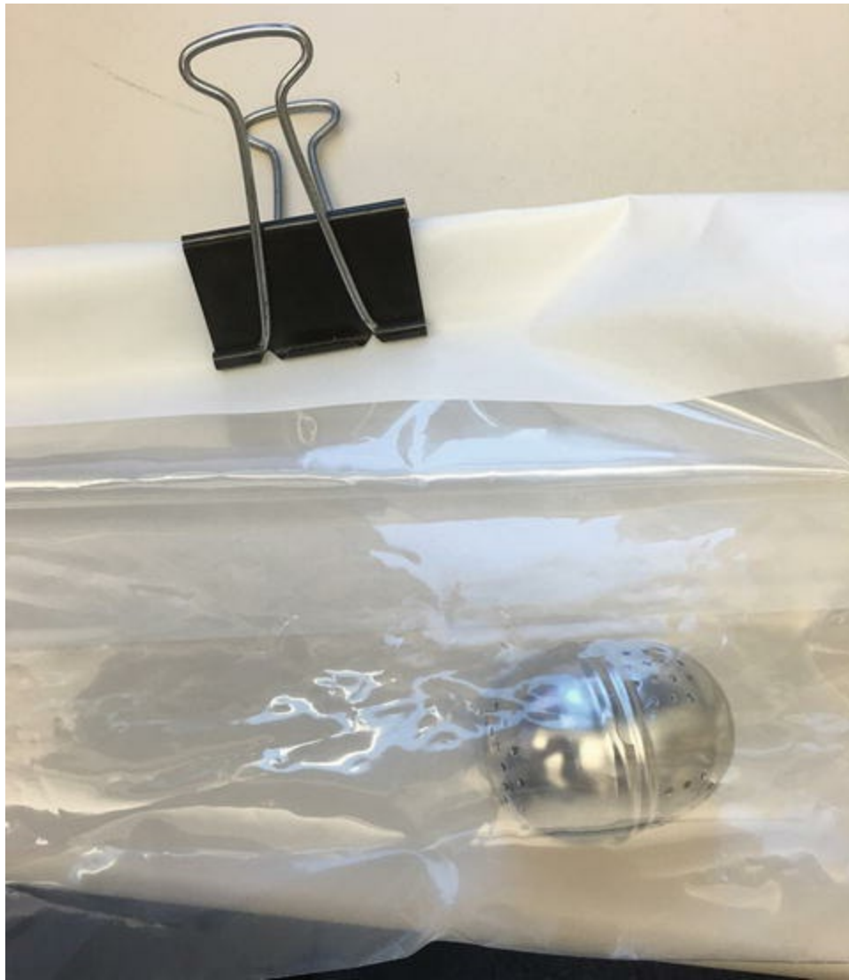
Fig. 3 A tea strainer fully charged with isoflurane inside 4 L Ziploc bag sealed with a metal clip
