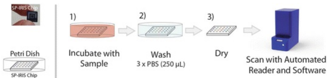
Fig. 1 SP-IRIS procedure flow. (1) Antibody-spotted SP-IRIS patterned chip is incubated with sample of interest. (2) Chip is washed and (3) dried. Finally, the chip is scanned. For procedural details, refer to Subheadings 3.2–3.4
