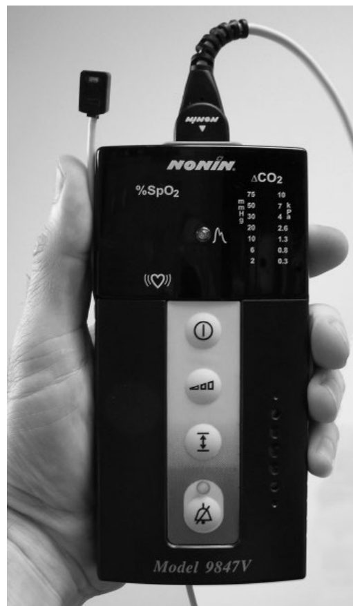
Figure 43.13 Portable hand-held monitor suitable for use as a pulse oximeter in detecting bowel viability (Nonin Medical, Plymouth, MN, USA). The reflectance sensor demonstrated or the clip-on sensors can be applied to the serosal surface of the bowel to obtain a rapid recording for blood oxygen saturation.
