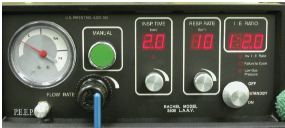
Figure 40.5 (A) Large-animal anesthesia machine from Mallard Medical (Redding, CA, USA) and (B) the ventilator control panel.
