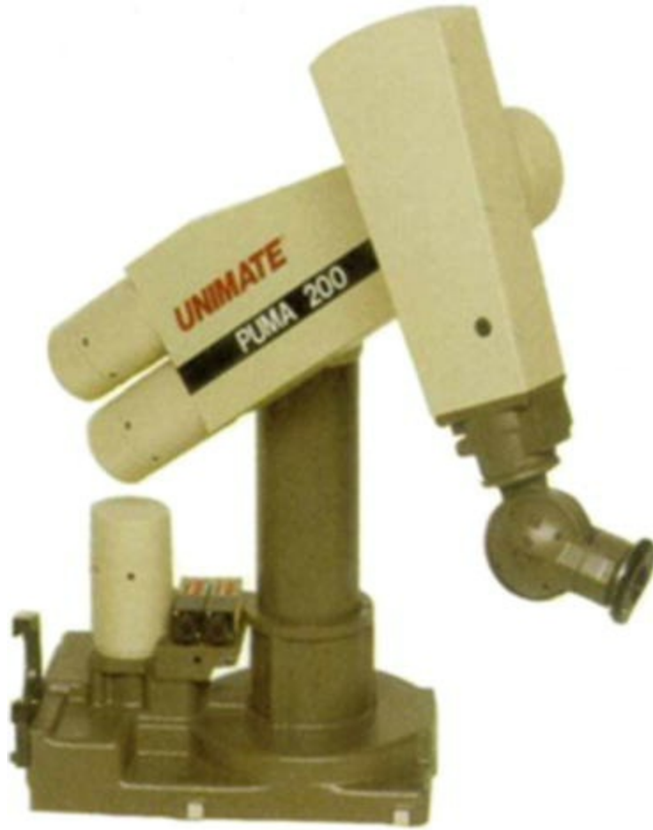
Fig. 20.2 Unimate PUMA 200 first robot used in a surgical intervention during a stereotactic brain biopsy
