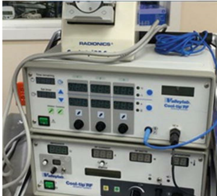
Fig. 16.3 The Cool-tip ® (Covidien, Valley Lab, Boulder, CO, USA) generator. System internally perfuses and chills each electrode to prevent charring of the target tissue; limiting the temperature increase to less than 25 °C
