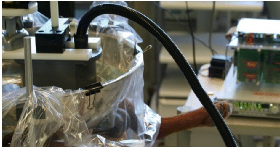
Fig. 23.2 The histotripsy transducer is positioned over the lower abdomen of a canine subject positioned supine. The focal volume of the transducer is co-localized within the prostate. A transrectal ultrasound probe is inserted in the rectum to provide imaging of the prostate and bubble cloud during
