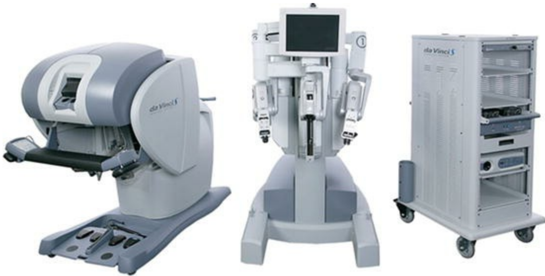
Fig. 20.8 The three components of the da-Vinci S (Intuitive Surgical, Sunnyvale, California), released in 2006: surgeon console, patient-side cart and the image- processing vision car
