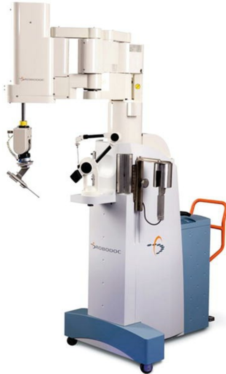
Fig. 20.3 ROBODOC used for the first time in 1988, during a total hip replacement
