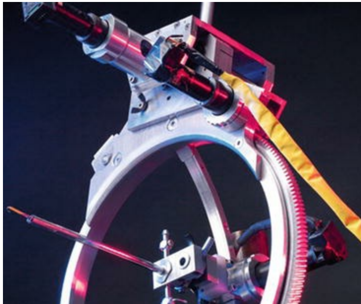
Fig. 20.4 The PROBOT was able to performed precise and repetitive cone shaped cuts of the prostate following a pre-establish plan
