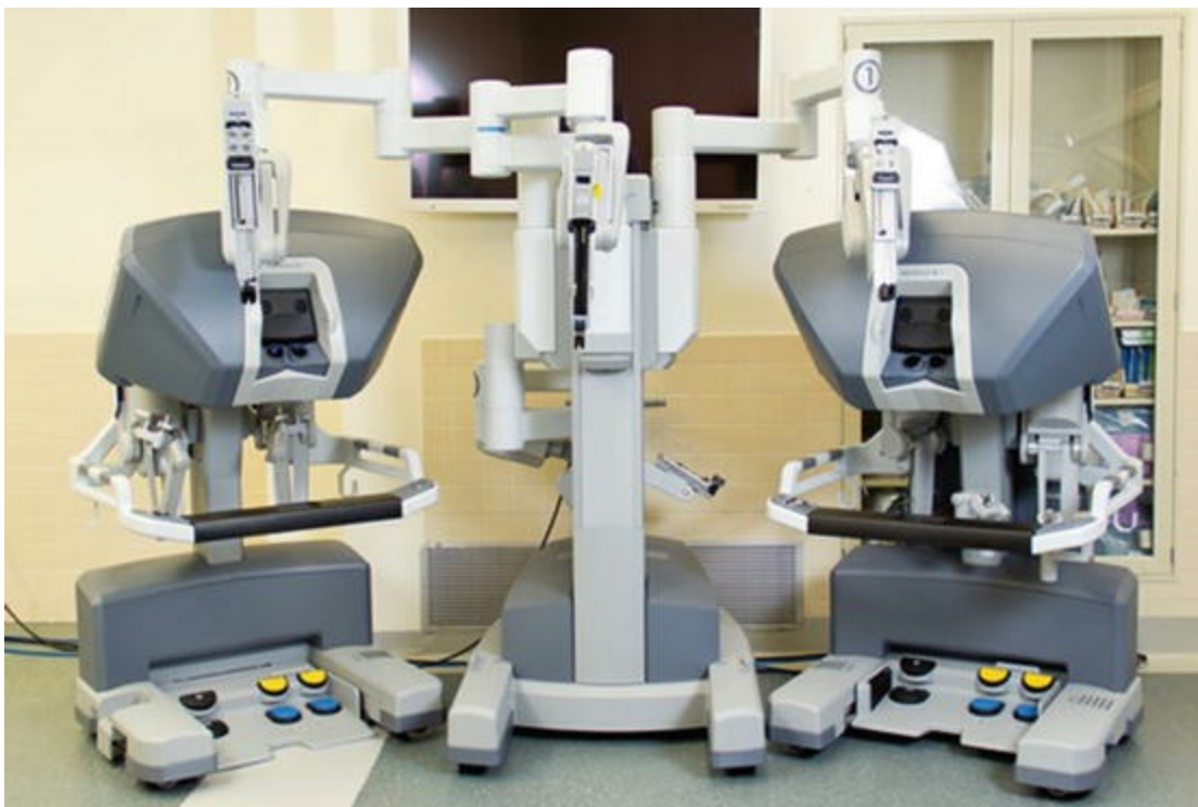
Fig. 20.9 The da Vinci Si dual console (Intuitive Surgical, Sunnyvale, California) allows a surgical mentor to teach with both the mentor and the trainee working at a surgeon console simultaneously
