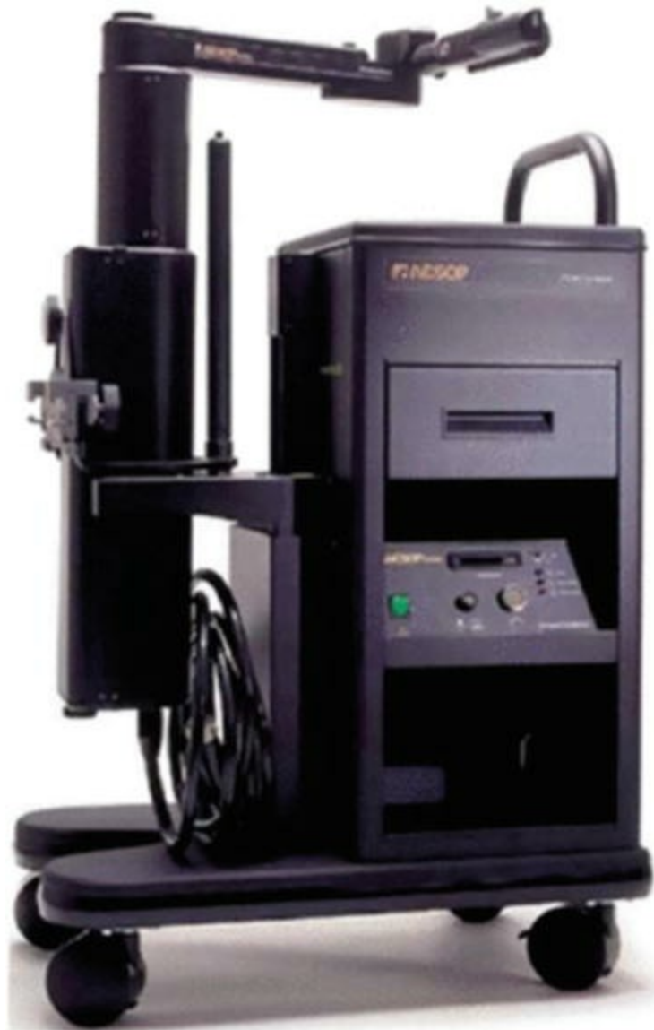
Fig. 20.5 AESOP ® (Automated Endoscope System for Optimal Positioning) , is a voice-activated robot used to hold the endoscope
