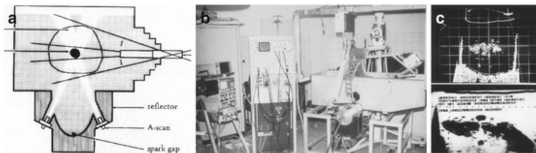
Fig. 11.4 (a) Integration of ultrasound scanners. (b) Experimental lithotripter with integrated ultrasound scanners. (c) Transverse sonogram after stone implantation
