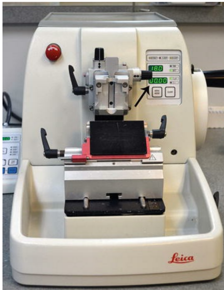
Fig. 11.8 An automated microtome is used for exhaustively sectioning through tissue blocks using systematic uniform random sampling (SURS) for stereology. After sections are collected at each sampling interval, the read-out on the microtome can be zeroed ( arrow ) and the block can be further sectioned until the next sectioning interval has been reached
