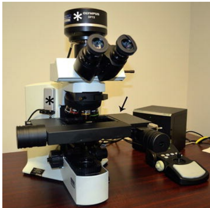
Fig. 11.12 Live microscope setup for stereology. The microscope contains a camera (white asterisk), motorized stage (arrow) and length gauge (black asterisk)
