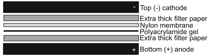
Fig. 5 The order of assembly for a dsRNA immunoblot transfer. From the bottom anode up, the stack should include a layer of extra thick filter paper, a nylon membrane, the polyacrylamide gel, and another layer of extra thick filter paper. The membrane and filter paper should be presoaked in transfer buffer ( 0.5\times TBE)
