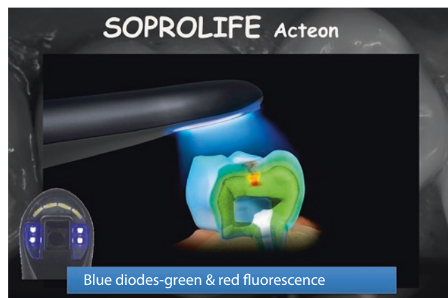
Figure 17.13 The SOPROLIFE light-induced fluorescence evaluator system uses in the blue fluorescence mode four blue LEDs emitting light at 450 nm. The light is transmitted through the enamel and then induces green fluorescence from the dentin body. If green light on the way back hits porphyrins in caries, the emitted fluorescence is red
