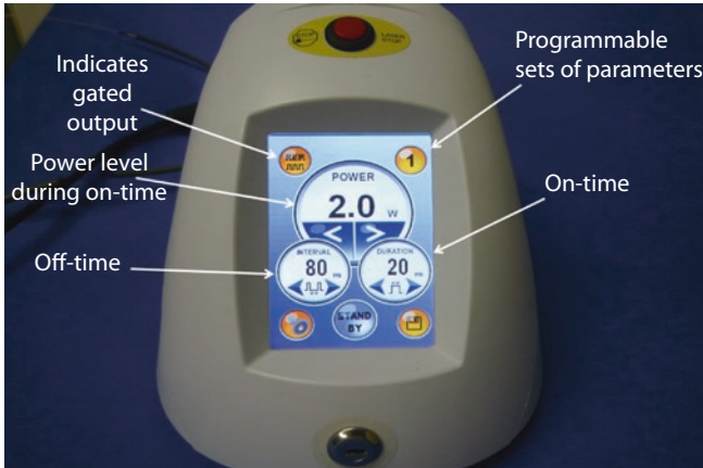
Fig. 4.27 This 810 nm diode laser has limited variables that may be controlled directly. It is used here with a 400 \mu\text{m} diameter optical fiber
