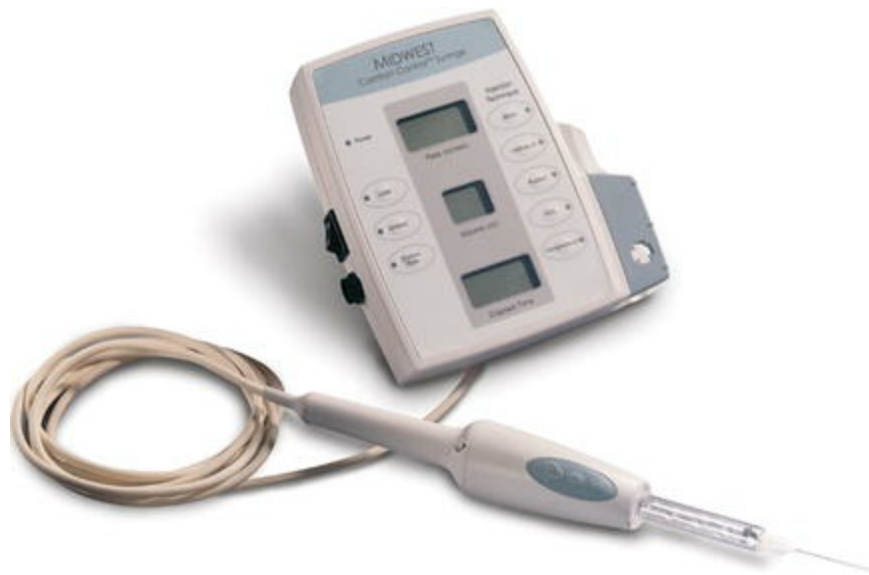
Fig. 8.5 The Midwest Comfort Control Syringe® consists of a control module and a handpiece with three buttons
