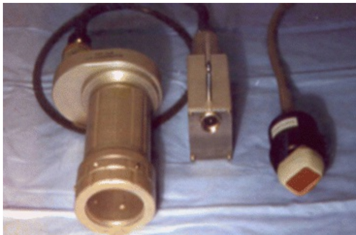
Fig. 1.16 Motorized device that housed an external stepper motor that mechanically rotated a built-in transthoracic transducer.
