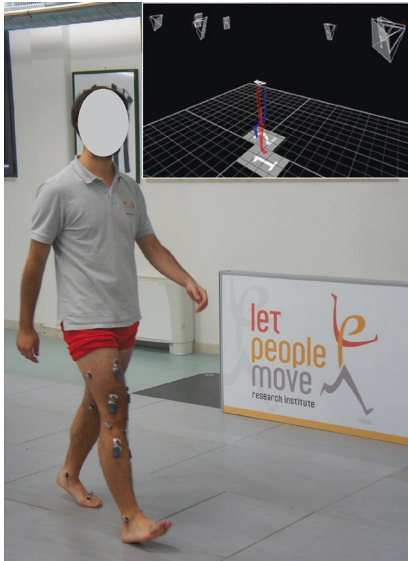
Fig. 38.3 Gait Analysis with 16-channel EMG telemetry and 3D systems
