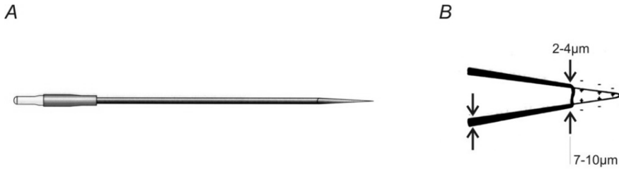
Fig. 6. Microneurography needle electrode. A shows a commercial tungsten needle electrode whose tip geometry is shown in B.
