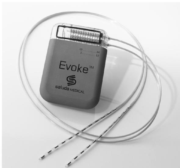
Fig. 2. An example implantable SCS device manufactured by Saluda Medical. This device is similar to other devices which are marketed in that it consists of a hermetic titanium implant which contains battery and electronics and this is connected to electrode arrays.
