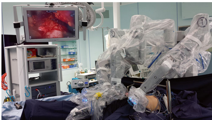
Fig. 11.15 Robot arms and camera docked in and positioned ready to start the rectus plication
