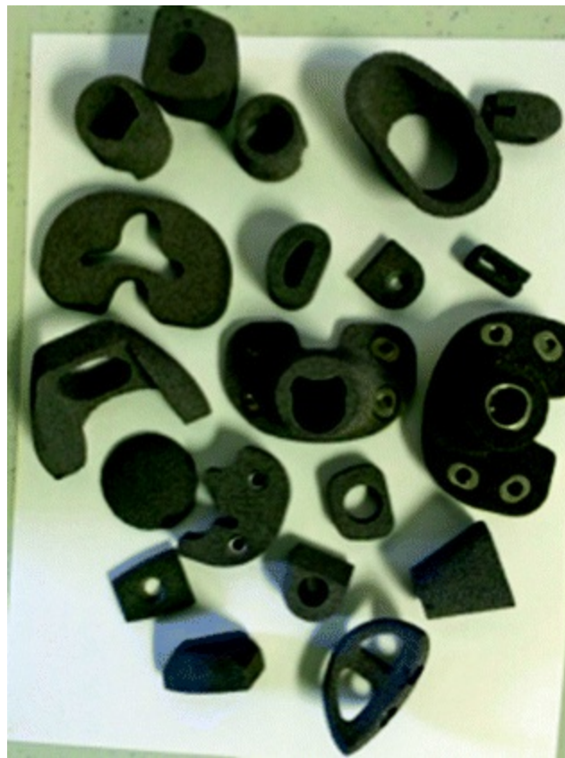
Fig. 15.9 Multiple different tantalum implants that can be fashioned for critical bone loss substitution
