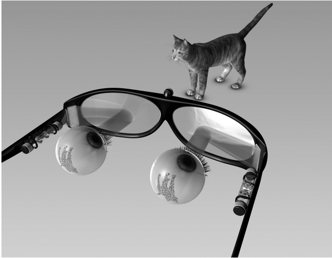
Figure 25.1 Holographic optical neural interfacing concept depicted in an illustration of the future optical-based prosthesis: the camera video stream is processed and fed to a holographic projection system. A spatial light modulator (placed in the corners of the glasses) phase modulates a laser beam wave-front and excitation patterns are projected onto the photosensitized retina. (A black-and-white version of this figure will appear in some formats. For the color version, please refer to the plate section.)
