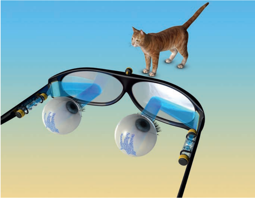
Figure 25.1 Holographic optical neural interfacing concept depicted in an illustration of the future optical-based prosthesis: the camera video stream is processed and fed to a holographic projection system. A spatial light modulator (placed in the corners of the glasses) phase modulates a laser beam wave-front and excitation patterns are projected onto the photosensitized retina.
