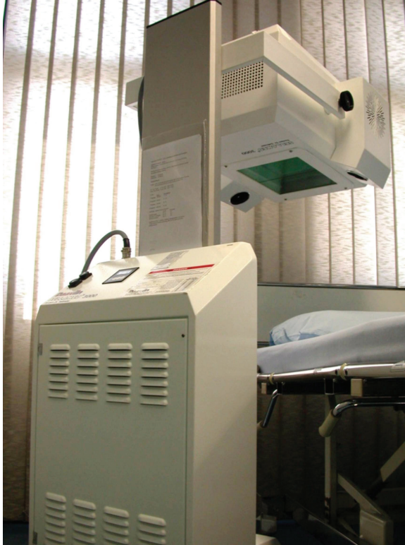
Figure 4. Localised flat-panel UVA-1 phototherapy unit.
