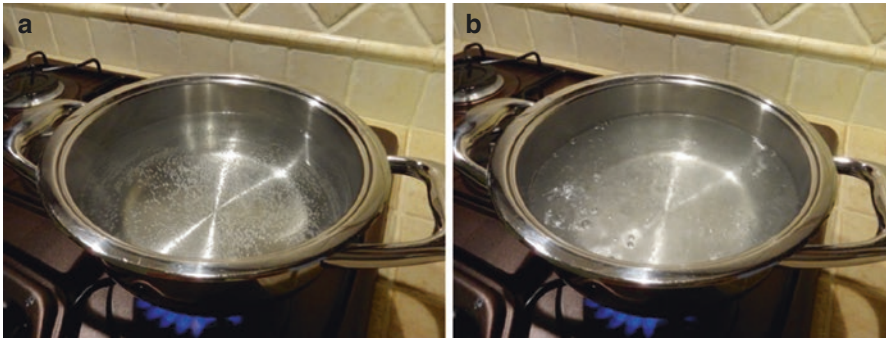
Fig. 4.2 A pot of water on the stove. (a) The water is not yet boiling but you can see many tiny bubbles. These bubbles are made of gases (mainly oxygen and nitrogen) which leave the solution due to their reduced solubility into water as temperature rises (dependence on temperature of Henry's law constant). (b) The water is now boiling (the bubbles are made of water)
