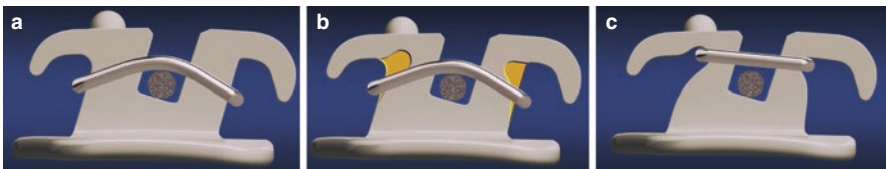
Fig. 7.8 (a) Conventional twin bracket. (b) Cutting the outer walls of the slot into slopes. (c) MLF bracket: the ligature wire is shifted up to increase the wire-slot clearance
