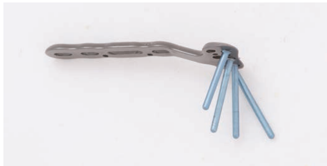
Figure 31.38 Deformed Volar locking plate
