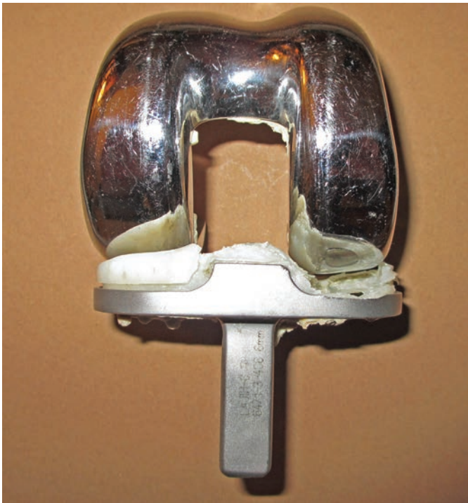
Figure 31.26 Anterior photograph of retrieval cruciate retaining (CR) total knee arthroplasty implant demonstrating catastrophic PE wear. The PE insert is generally more flat to allow femoral rollback onto the posterior part of the bearing
