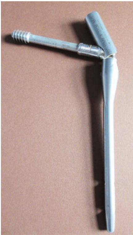
Figure 29.7 (a, b) Photographs of retrieved broken IMHS
