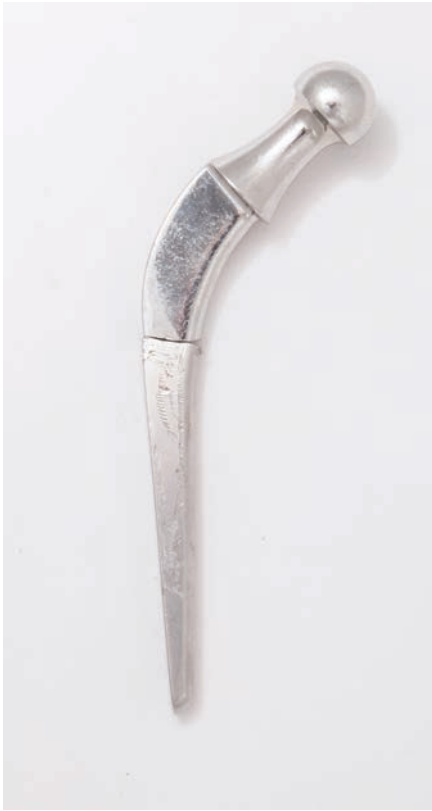
Figure 31.21 Photograph of stem retrieval due to stem fracture
