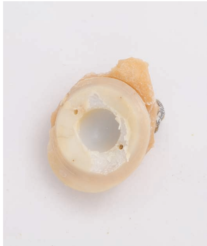
Figure 31.27 Photograph of retrieval acetabular cup implant demonstrating cracking and delamination of its edge from neck impingement
