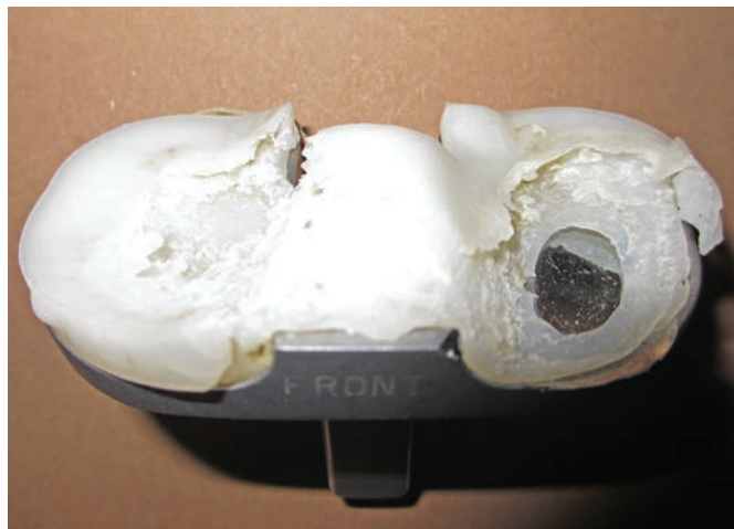
Figure 31.25 Photograph of retrieval tibial knee implant demonstrating catastrophic PE wear
