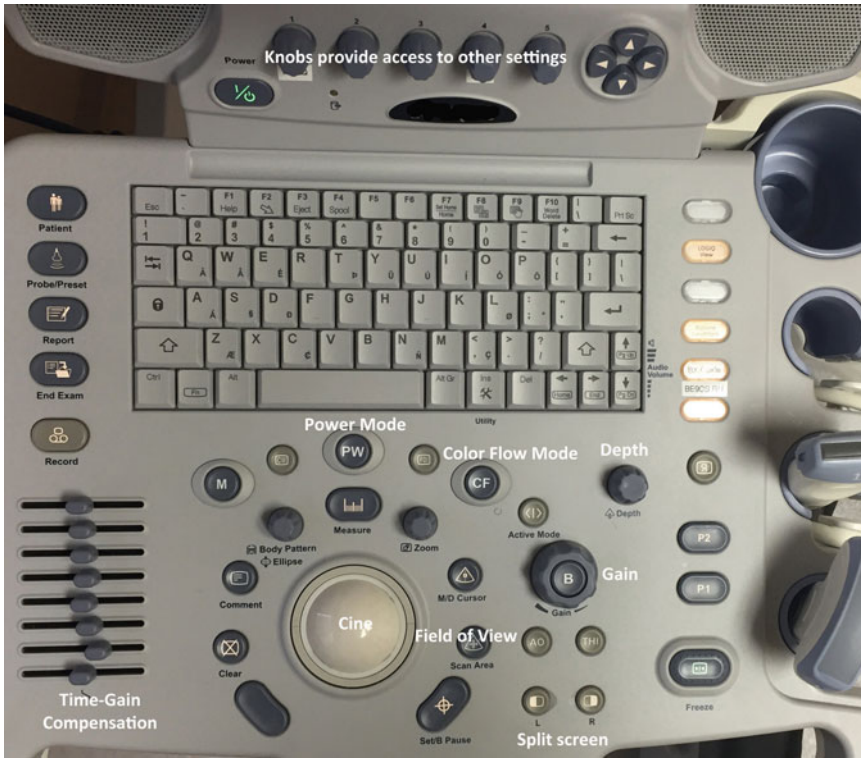
Fig. 4.7 A typical console interface showing common user-controlled variables
