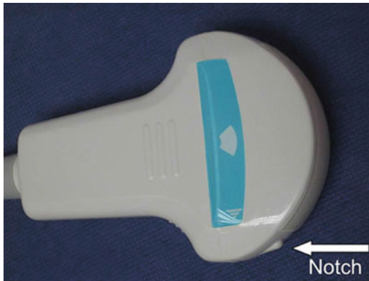
Fig. 8.3 Curved-array transducer with orienting notch (arrow). The notch is, by convention, oriented to the patient’s head during longitudinal scanning and to the patient’s right during transverse scanning
