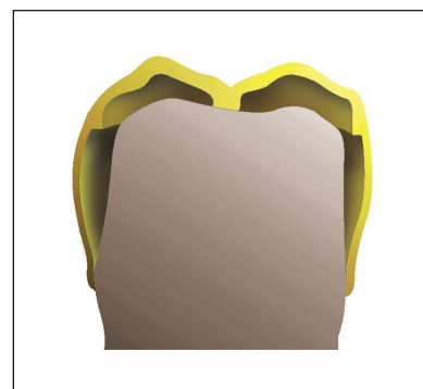
Fig 2-95 The cast occlusal surface is soldered to the ring. An occlusal stop is placed to avoid displacement of the crown.
