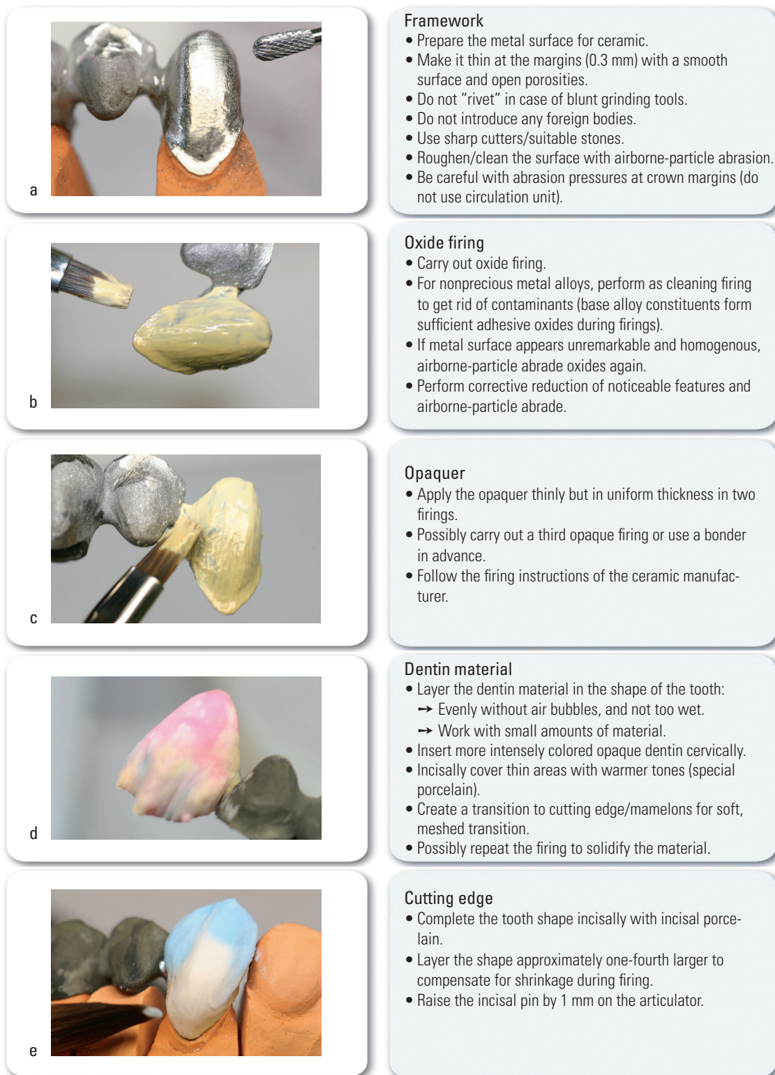
Fig 5-78 Ceramic veneering. (a) Prepare the framework of a veneer crown. (b) Carry out oxide firing. (c) Apply/fire the opaquer. (d) Apply/fire the dentin material. (e) Layer/fire the cutting edge.
