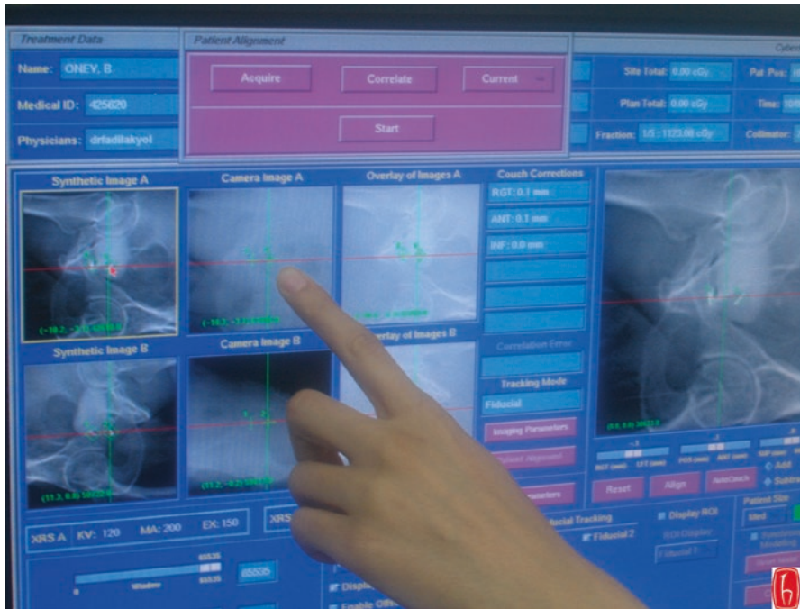
Fig. 18.7 Daily kV imaging of gold fiducials for rSBRT
