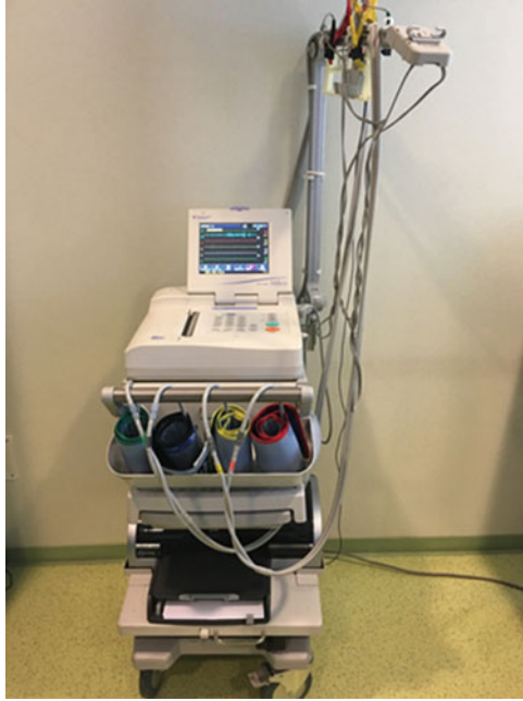
Fig. 2.39 VaSera ® VS-1500 and VS-2000 (Fukuda Denshi, Japan)—Fukuda suggests cardio-ankle vascular index (CAVI) as an index for the measurement of arterial stiffness. Unlike the instruments using the brachial-ankle pulse wave velocity system, the VaSera ® uses the recording of cardiac tones as a central reference point for the assessment of pulse wave velocity. As for peripheral recording, a cuff is placed at the ankle, which records pulse wave using an oscillometric method. Therefore, this system records the distensibility of the whole aorto-iliac, femoral-tibial segment. This system, as well as the brachial-ankle pulse wave velocity systems, considers both the aorta and the peripheral arterial axis of the lower limb, but this can lead to incorrect definition of aortic distensibility
