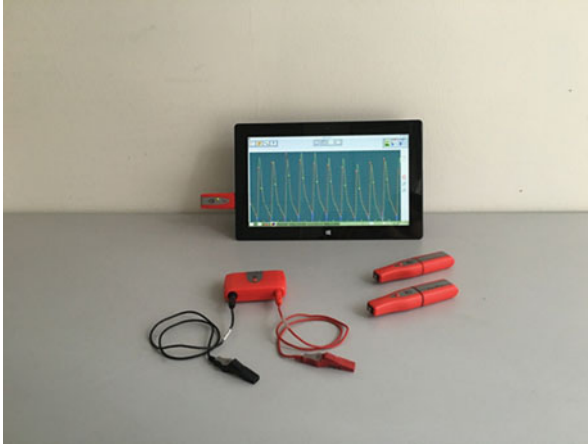
Fig. 2.31 The PulsePen ® WPP-ETT (DiaTecne srl, Italy)—This model of PulsePen ® (WPP-ETT) measures carotid–femoral PWV at one time by using two high-fidelity tonometers [15]. The proximal tonometer is placed on the common carotid artery and the second tonometer records the pulse wave curve simultaneously in the peripheral artery. It is a pocket-size wireless sympathetic system composed of a receiver, an optional table-PC, two tonometers, and an electrocardiograph. The recording of the ECC tracing allows the measurement of carotid–femoral pulse wave velocity also at two times by using one tonometer combined with electrocardiographic tracing. This method is suitable when the test is carried out only by one operator, namely when the recording of the two arterial signals could be difficult. High-fidelity tonometers are very sensitive and pressure waveforms are generally acquired easily; femoral pressure waveforms can be recorded by placing the probe on clothing (even on blue jeans), and patients do not need to undress in most cases. The whole test usually lasts from 4 to 8 min. At the end of it, an automatic report can be printed for the patient. The PulsePen ® is available in anthracite gray and Ferrari red, symbol of Italian technology and design. The recording of pulse wave velocity and central arterial pressure is a real fun!
