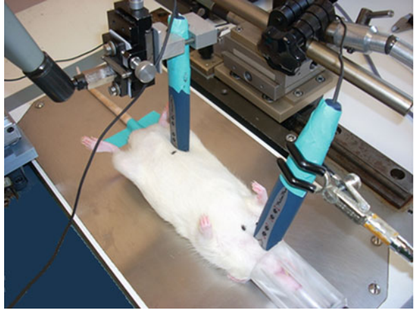
Fig. 8.2 Non-invasive assessment of carotid–femoral pulse wave velocity in a spontaneous hypertensive rat. Arterial pressure waves are simultaneously recorded in carotid and femoral arteries with PulsePenLab ® arterial tonometer
