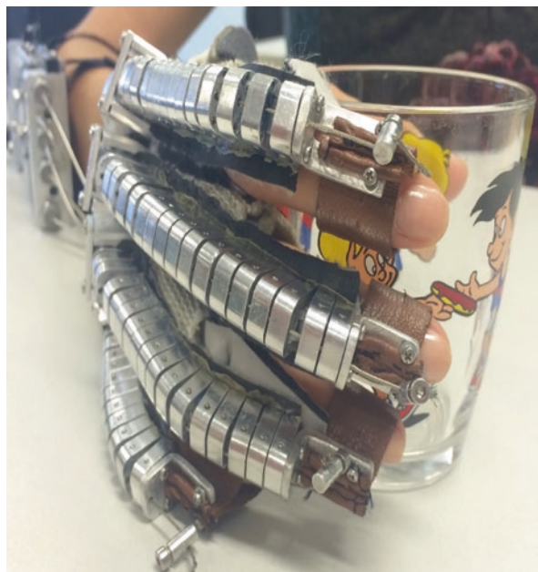
Fig. 19.4 Fingers Extending eXoskeleton (FEX) for rehabilitation and regaining mobility (Patent: PCT/IB2015/059313)
