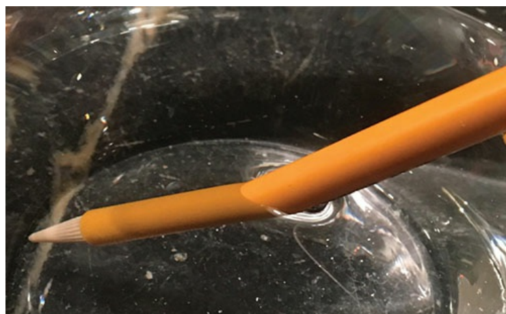
FIGURE 13-5 Effect of refraction as light moves from materials of different indices of refraction.
