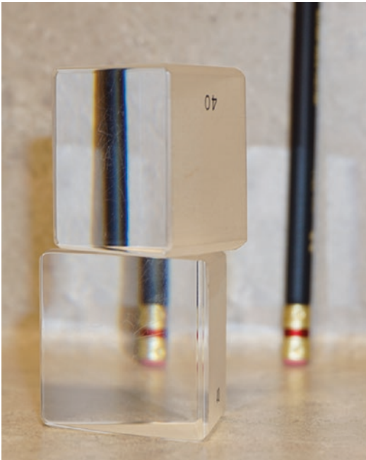
Fig. 2.3 Two 40 \Delta prisms are stacked with the back surfaces not parallel. The orientation of the back surface influences the effective power of the prism, as evidenced by the pencil's image being displaced differently through the two identical prisms
