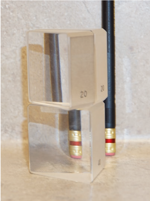
Fig. 2.2 On the bottom is a 40 Δ prism. On top of that is a sandwich of two 20 Δ prisms. The top prism sandwich has a much greater value than the 40 Δ prism, as evidenced by it displacing the image of the pencil much further
