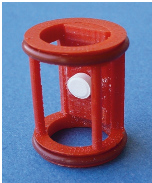
Fig. 1 Image of 3D printed holder with mounted tablet containing BAT
