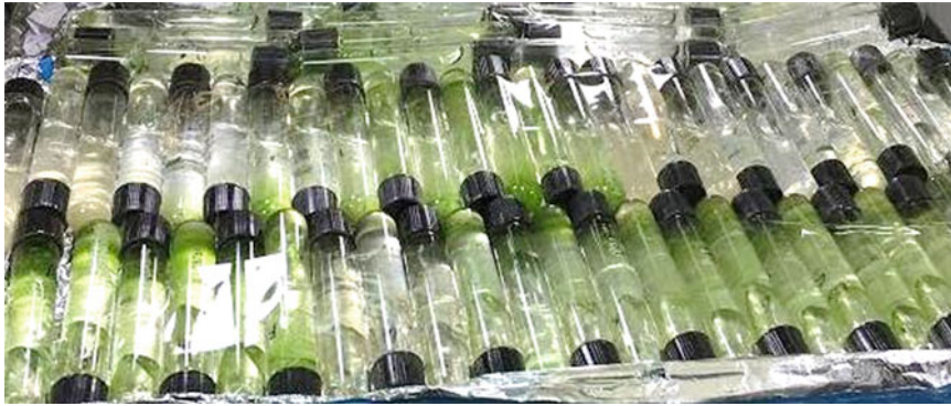
Fig. 1 Microalgal toxicity assay using Chlorella sp. performed in screw capped glass tubes
